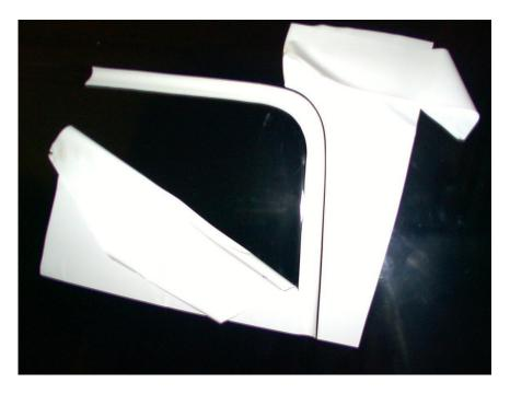
1 Apply VWS over the panel and recess. Cut a strip of the film (fillet) wide enough to fit into the recess and internal edges allowing material for trimming. Remove the excess material leaving the fillet. Working from the centre of the recess outwards in both directions, squeegee the vinyl into the base of the recess, around the internal radii and up to the outside edges of the recess. Remove the waste from the panels.
