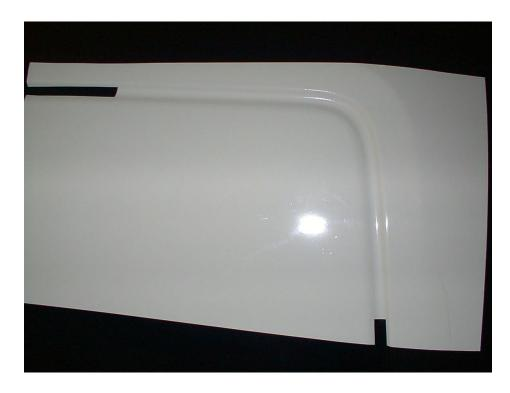
3 Demonstration of a completed recess corner. Some material has been removed from the recess for clarity.
