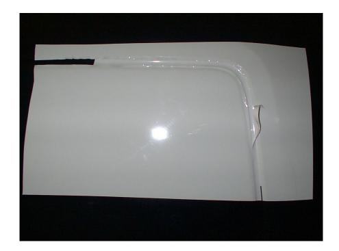
2 Apply VWS to the flat panels and cut to overlap the edges of the vinyl in the recesses. Use gentle heat if necessary on the corners. This application method hides the joint line from view and ensures that the vinyl remains in the recesses.
