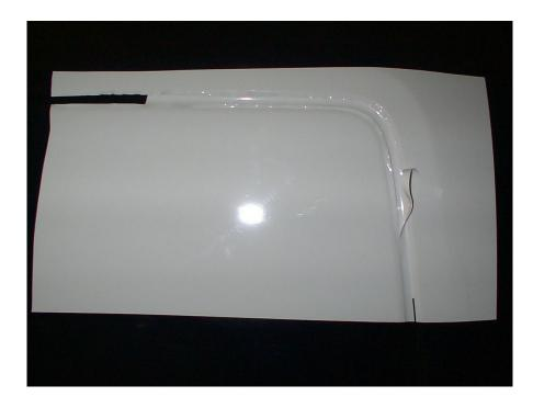
Apply VWS to the flat panels and cut to overlap the edges of the vinyl in the recesses. Use gentle heat if necessary on the corners. This application method hides the joint line from view and ensures that the vinyl remains in the recesses.
