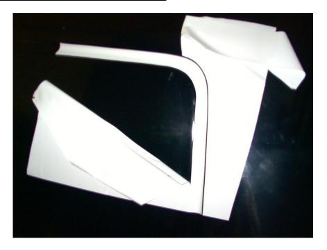
Apply VWS over the panel and recess. Cut a strip of the film (fillet) wide enough to fit into the recess and internal edges allowing material for trimming. Remove the excess material leaving the fillet. Working from the centre of the recess outwards in both directions, squeegee the vinyl into the base of the recess, around the internal radii and up to the outside edges of the recess. Remove the waste from the panels
